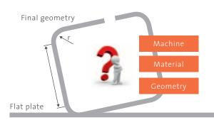
Multi Radial geometries such as ovals, cases or buckets are obviously challenging objectives for plate roll operators. However, the lucky operator who can rely on BENDtronic is also "in good shape" here. After the graphically supported definition of the final geometry, BENDtronic calculates the machine settings and all the steps from the flat plate to the final geometry. The operator can start rolling right after the process simulation.
